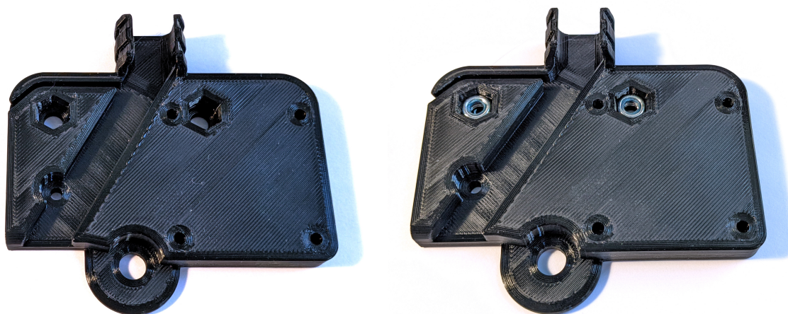
Figure 1.5: Press the M5 locknuts into the holes in the main mounting plate
